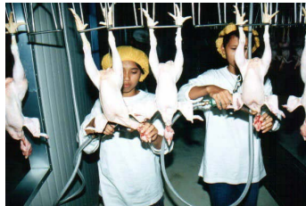
Neck cutting with an air-powered scissor
